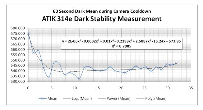
The camera seems to take from  $T_0$  to  $T_5$  to get to temperature but the oscillations do not settle out until around  $T_{15}$ . Cooling was in effect from approximately  $T_0$  to  $T_{27}$ . The mean data as recorded:
