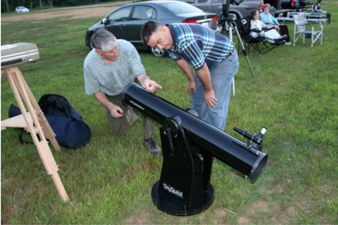
Joe and Ranny using a Laser Collimator to align the primary mirror
